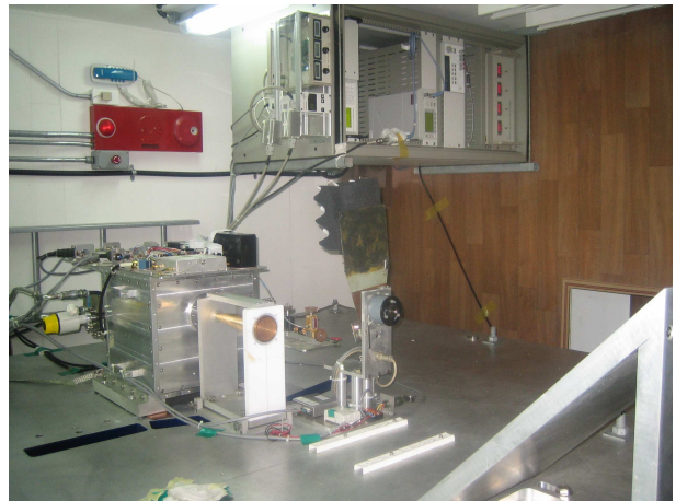
Fig. 2. — Inside the receiver room of the KVN Ulsan radio telescope, which is pointed to the zenith. The 100-GHz band receiver is seen with the feed horn on the receiver plate, while the 45^\circ mirror is on the right bottom corner. The vertex window is above the mirror.
